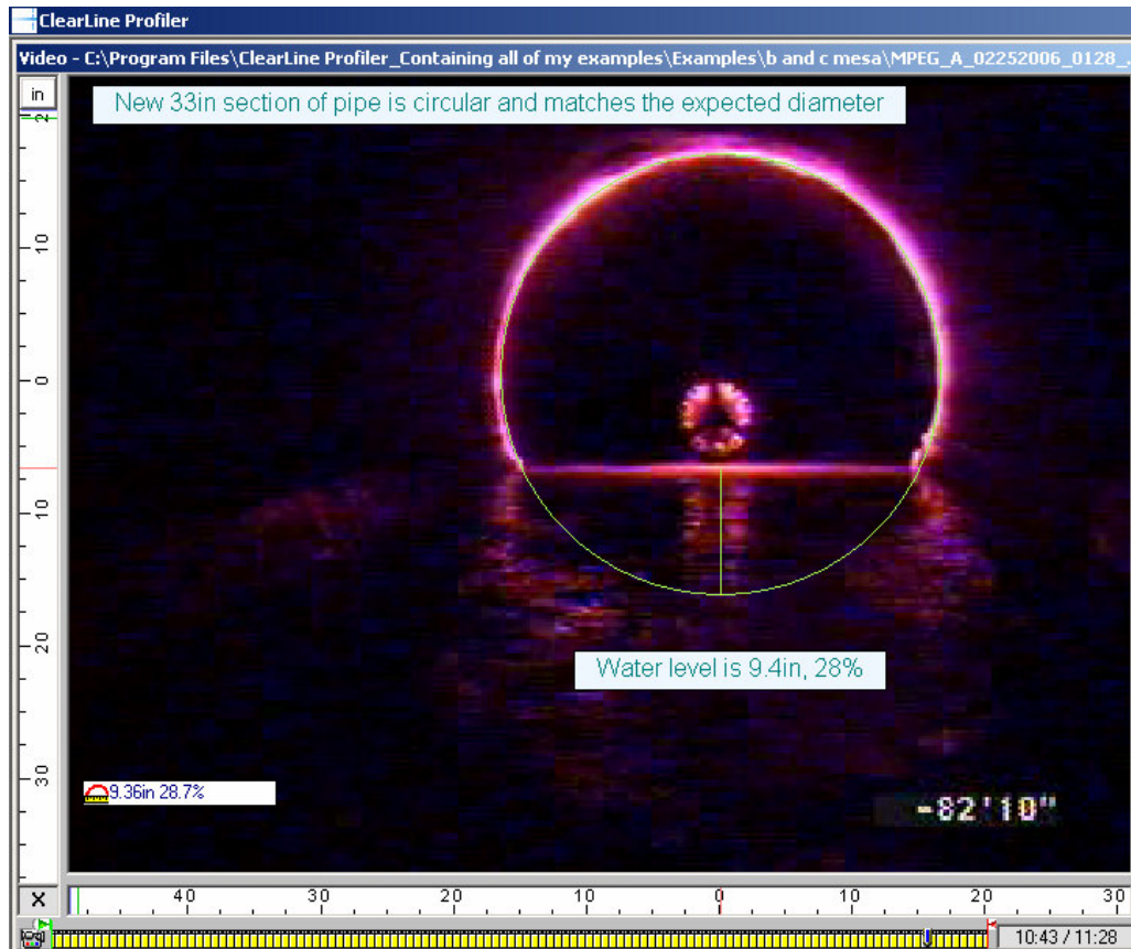
Figure 2: The profiler setup verified and the water level is about 28% for the line.
