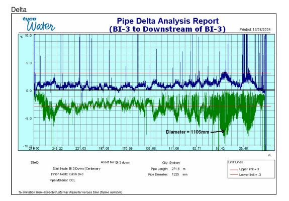
Similar levels of compression are evident from 23m (25.25m) through to 16m (18.25m).
