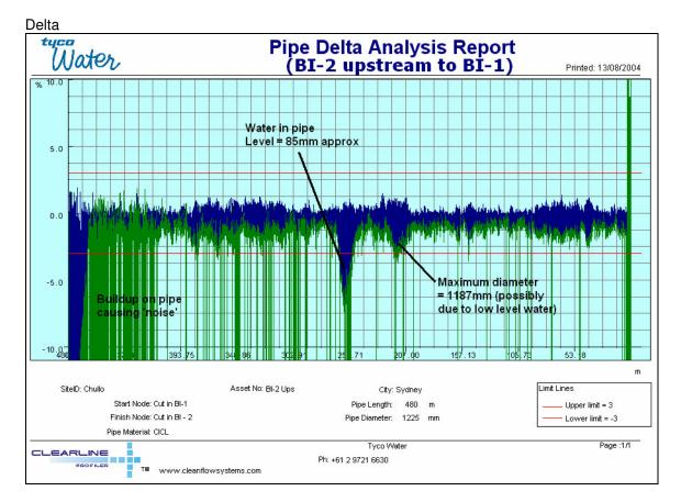
There is a dip of 85mm (water level) in the pipe at 286m (288.25).
