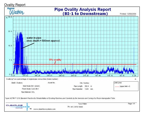
There is water in the pipe from 346m (348.25) and increases to a maximum level of approximately 500mm at 391m (393.25) downstream of BI-1. At this point, the high water level stops the profiling from continuing. This indicates a significant dip in the pipe.
